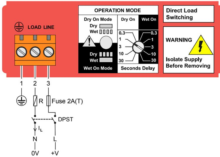
R = External load (must be fitted)
