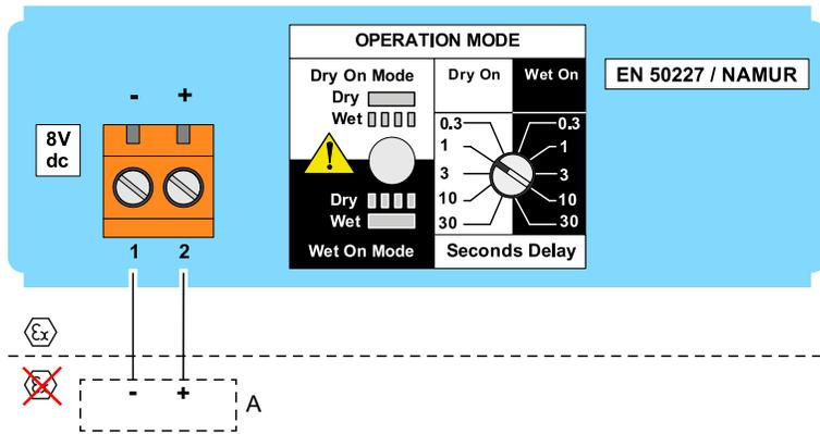
A. A certified intrinsically safe isolating amplifier to IEC 60947-5-6
