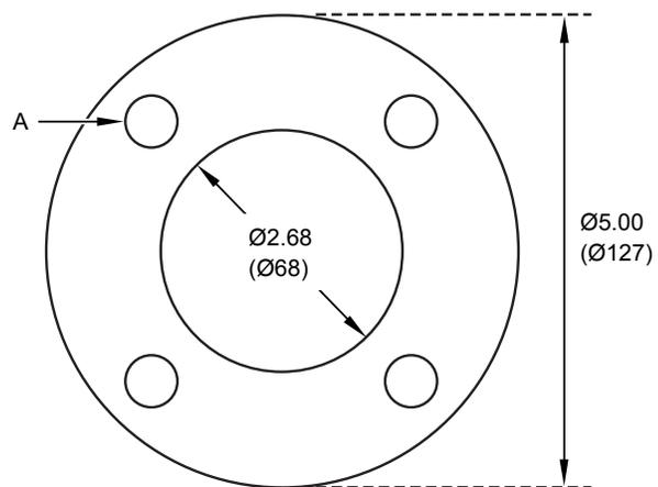
A. 4 off  $\text{Ø}0.55$  ( $\text{Ø}14$ ) holes equi-spaced on 3.97 (98.4) PCD
