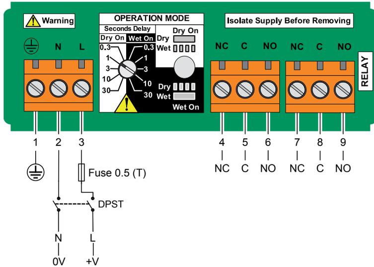
Figure 7: Relay DPCO Cassette, 12 Vdc Nominal Version (Green Label) – Code E
