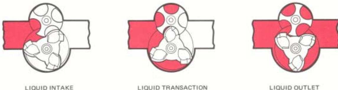
Figure 1 - BiRotor Meter Principle of Operation Diagram
