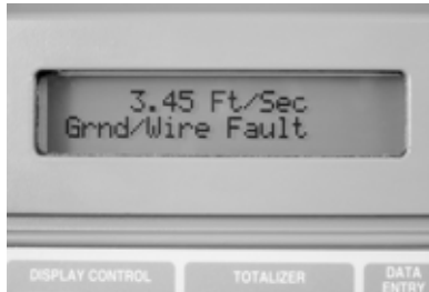
Grounding and wiring fault displays on LOI.
