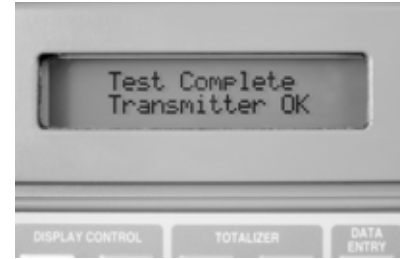
Transmitter Calibration is verified.
