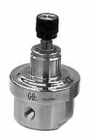
The PR-7ULF Series pressure reducing regulator is designed to furnish ultra precise low outlet pressure control to analytical instrumentation. With the combination of the large diaphragm sensing area of the PR-7 Series regulator and a super low flow valve seat assembly, pressure control down to 1 inch of water at 2cc of flow is easily obtainable.
